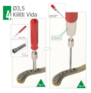
\*Send Ø3.5 mm locking screw with Ø 2.5 mm allen screwdriver. (1.5Nm torque) .(Fig.17-18)
